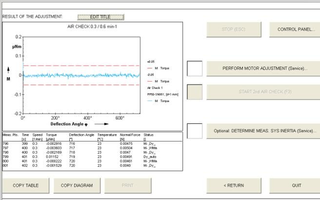
Fig. 2: Example of an air measurement with limit values
